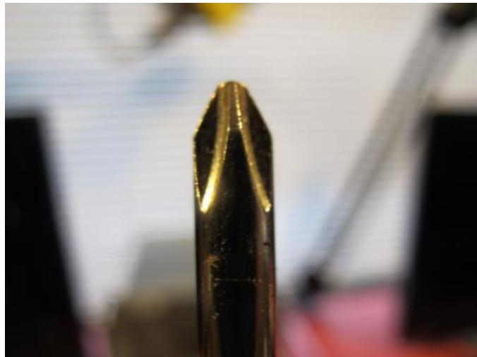
Let's say you have a badly rusted Phillips (or similar) screw that you need to remove. Don't just push the screwdriver into the rusted head and hope for the best. First, get a pick with a fine point and work the rust out of the screw head. Blow it out and scratch some more. Scratch until you're removed as much rust that is going to come out. THEN put your screw driver into the screw. MUCH more grip. Once you've "cammed out" the screw head, you're doomed. Scratch the rust out before you even try.
